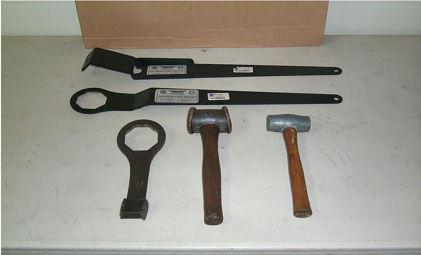
EAR TYPE KNOCK-OFF TOOL: OCTAGON KNOCK-OFF TOOL: OCTAGON KNOCK-OFF ADAPTOR (FACTORY TOOL PART # HAC67): HEAVY DUTY COPPER HAMMER: LEAD HAMMER:
