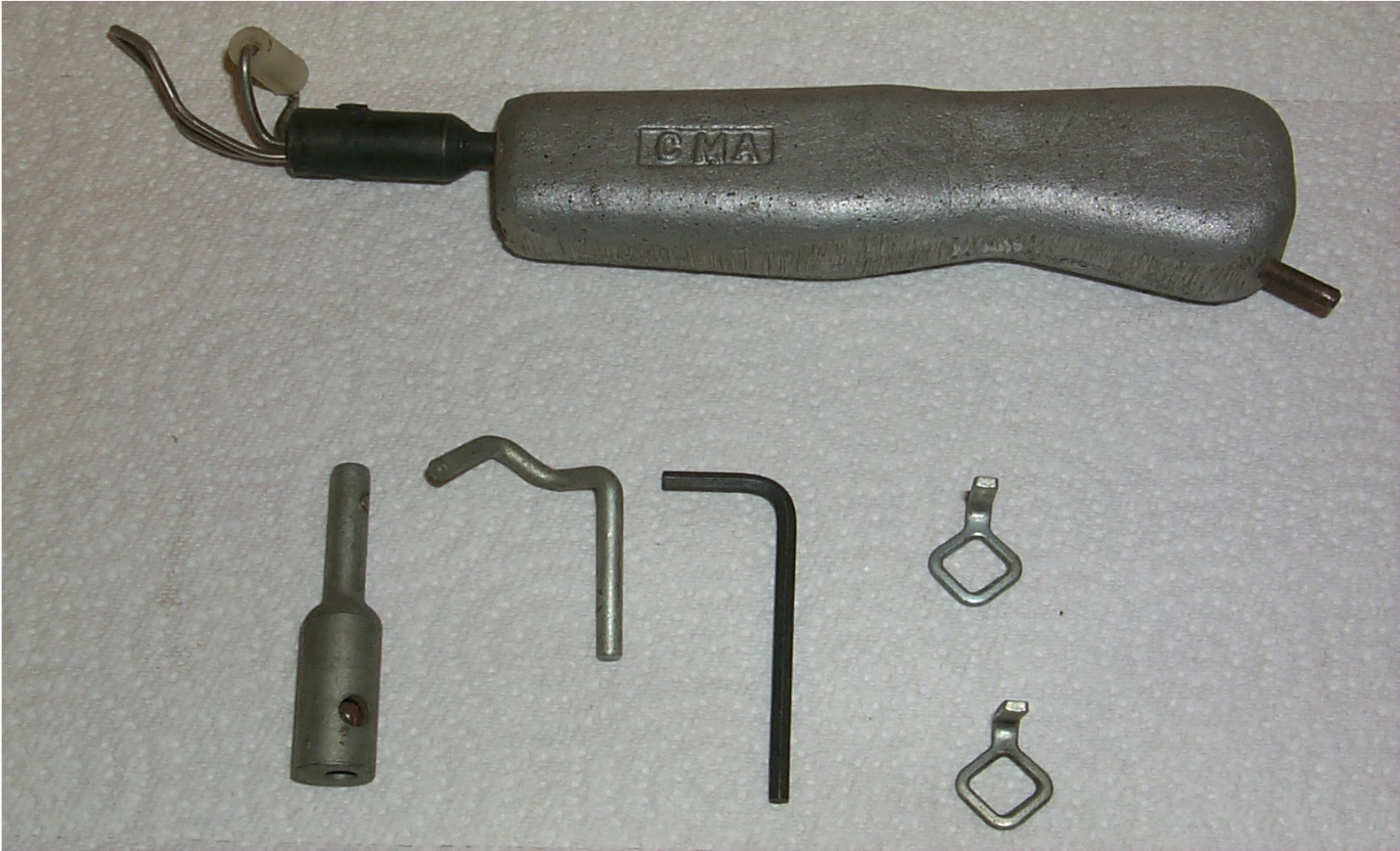
THIS TOOL 18G468/JD23 IS USED FOR INSTALLING THE RUBBER EXPANDER SEALING STRIP ON WINDSHIELDS
