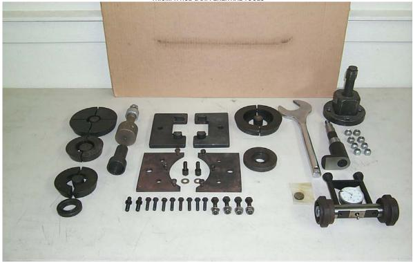
1st ROW (TOP TO BOTTOM) SHOWS THE VARIOUS ADAPTORS THAT ARE USED WITH MASTER TOOL SHOWN IN IMAGE P0004010 (MASTER TOOLS AND TOOL CATALOG FOLDER): 18G47BD (TRIUMPH MODELS AS WELL AS JAGUAR MG & LAND ROVER MODELS): BLT2051/S4221A-16 (TRIUMPH MODELS): BLT2052/S4221A-17 (TRIUMPH MODELS AS WELL AS MGB & JAGUAR MODELS):
