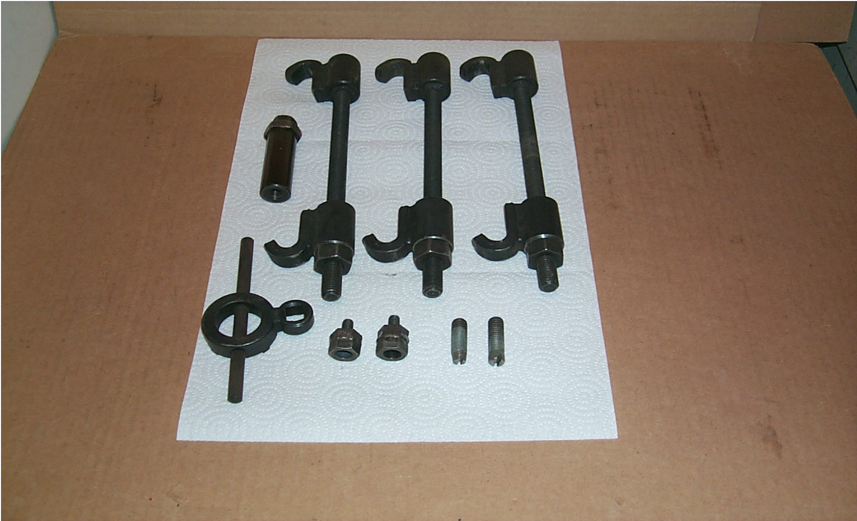
CYLINDER HEAD STUD REMOVAL TOOL (S350/1 CHURCHILL): FRONT STRUT COIL SPRING COMPRESSOR (BLT2074): FRONT STRUT CLOSURE NUT REMOVAL TOOL (RTR359): WATER PUMP REMOVAL ADAPTOR x 2: CYLINDER HEAD GUIDE STUDS x 2:
