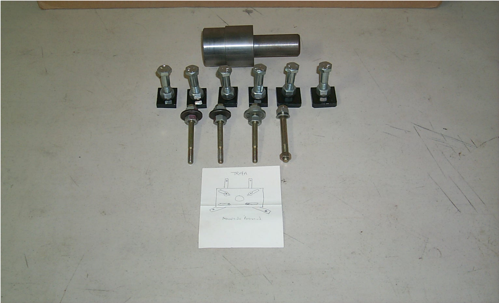
TR4A REAR MAIN CRANKSHAFT HOUSING CENTRALIZER: CYLINDER SLEEVE RETAINERS: ENGINE MOUNTING STAND HARDWARE & DIAGRAM (USE WITH ENGINE ASSEMBLY STAND). SEE ENGINE STANDS IN "BA TOOL & EQUIPMENT SALE IMAGE" FOLDER
