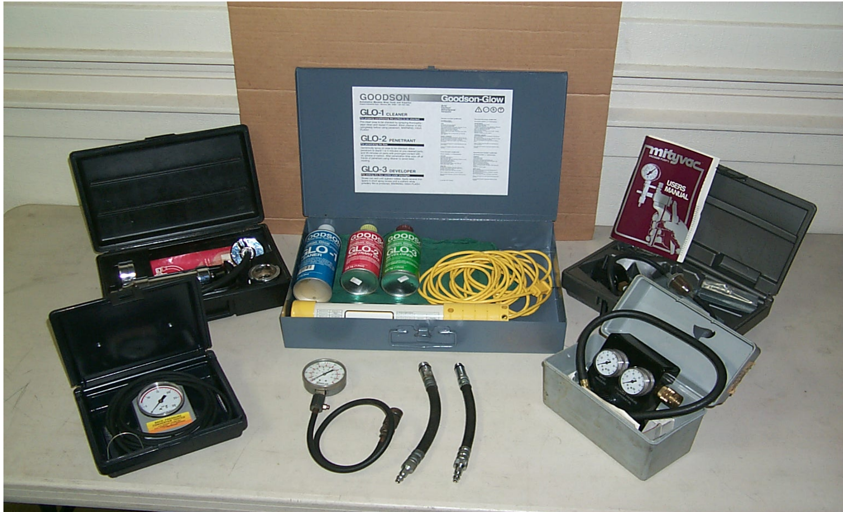
RADIATOR PRESSURE TESTER: CYLINDER HEAD & ENG BLOCK CRACK TESTER: VACUUM HOLD TESTER: EXHAUST BACK PRESSURE TESTER: COMPRESSION GAUGE (14mm & 18mm ADAPTORS): CYLINDER LEAK DOWN TESTER:
