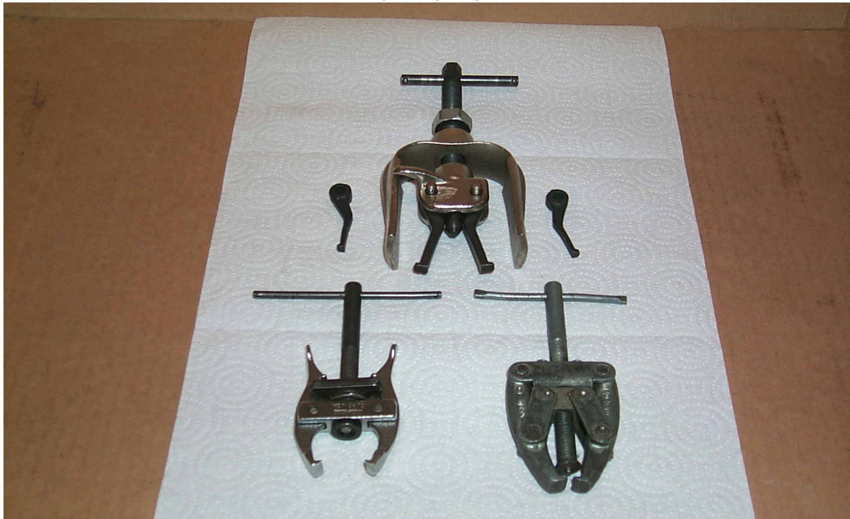
VARIOUS SIZED PULLERS FOR AN ASSORTMENT OF USES. NOTE: THE UPPER PULLER CAN BE USED FOR REMOVING THE MGB CRANKSHAFT BUSHING (SHORT TYPE)
