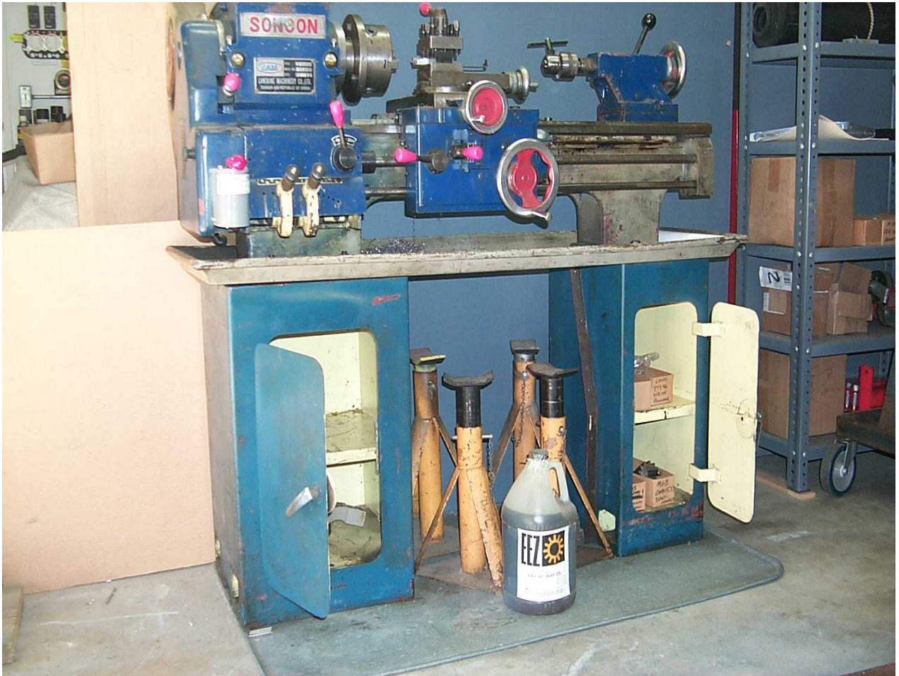
SONOON LAM10X36 350B LATHE 3 JAW CHUCK WITH ACCESSORIES (CIRCA LATE SIXTIES LATE SEVENTIES ?) ELECTRIC MOTOR 115/208-230 VOLTS: 1 HP: 60 HERTZ: 1730 RPM
