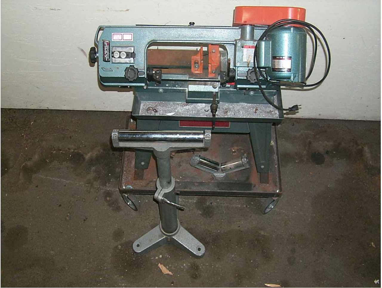
MOBILE BAND SAW WITH ROLLER STANDS (115/230 VOLT MOTOR SINGLE PHASE):
