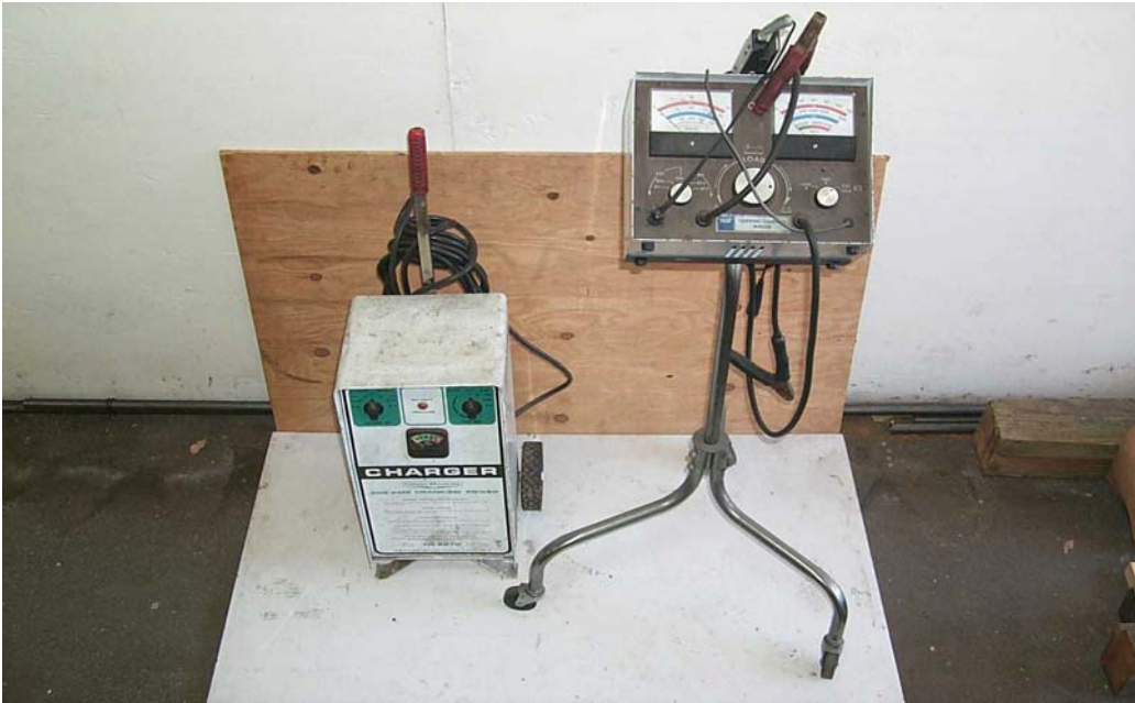
HEAVY DUTY BATTERY CHARGER/STARTER (300 AMP CRANKING POWER) CARBON PILE BATTERY TESTER & CHARGING CIRCUIT TESTER
