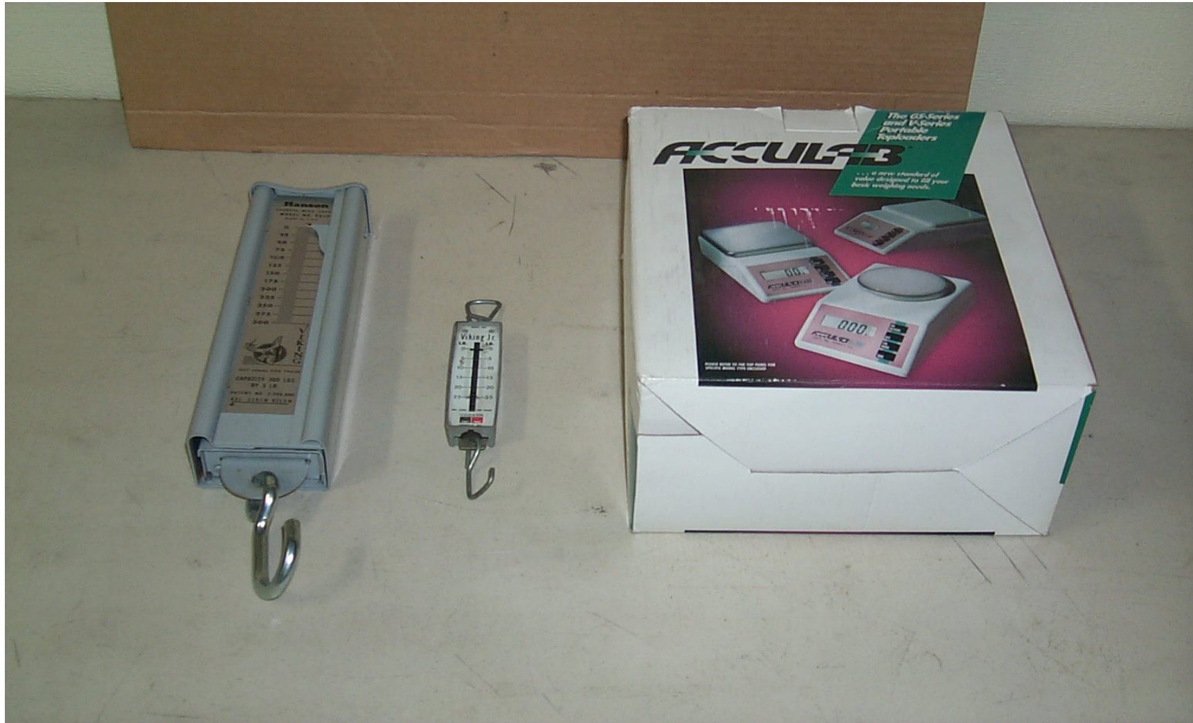
HEAVY DUTY PULL SCALE (0-300 LB): LIGHT PULL SCALE (0-25 LBS): TABLE SCALE (0-6000G):
