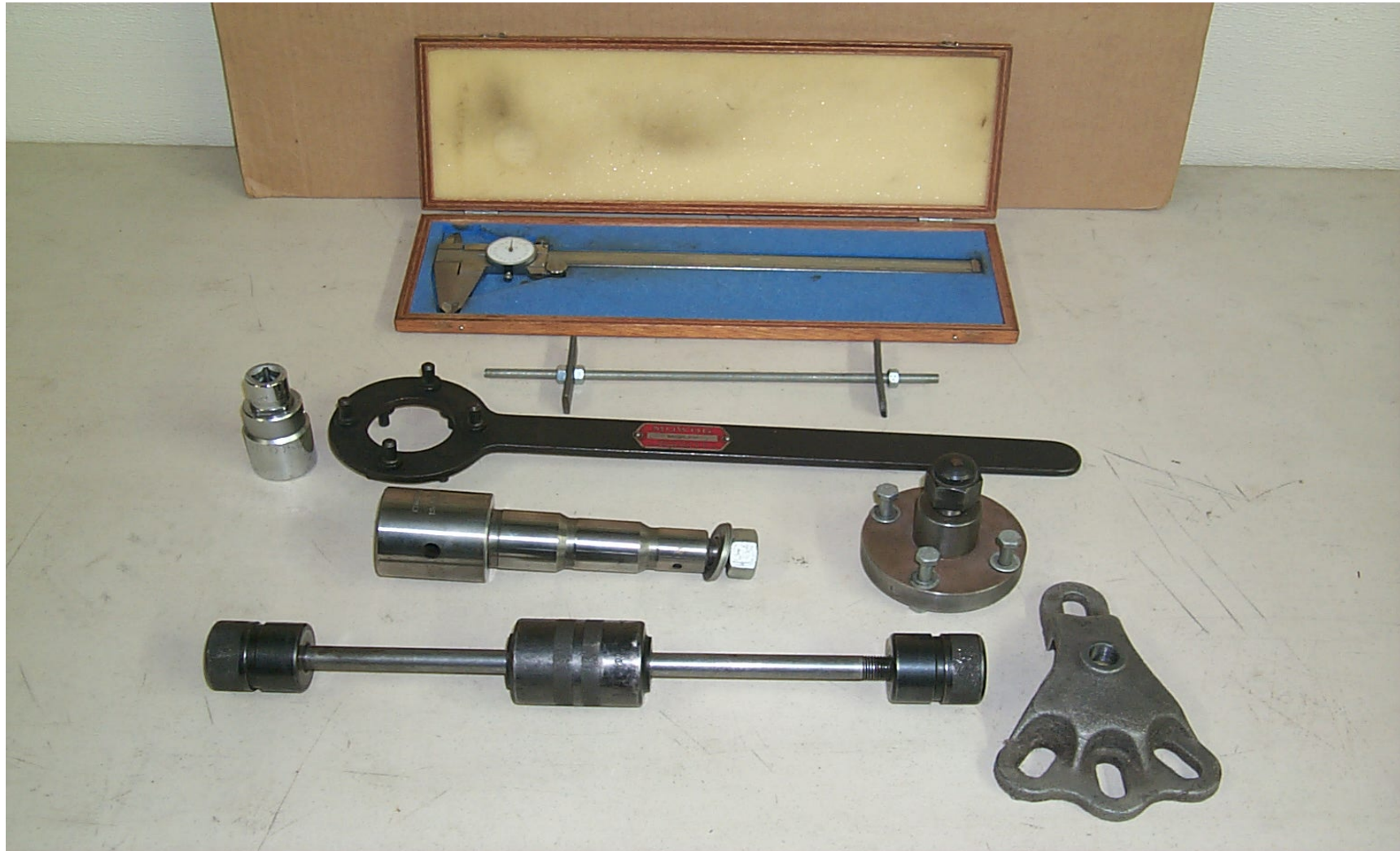
12" DIAL CALIPER GAUGE WITH ADAPTOR TOOL (USED FOR MEASURING WIDTH OF CROWNWHEEL ASSEMBLY): PINION FLANGE NUT SOCKET (1/2" DRIVE ADAPTOR): PINION FLANGE HOLDER 18G34A: DUMMY PINION 18G191H/I: PINION FLANGE REMOVER: FACTORY SLIDE HAMMER 18G284 (AXLE SHAFT REMOVER MGB TUBE AXLE): HUB ADAPTOR (BANJO AXLE HUB):
