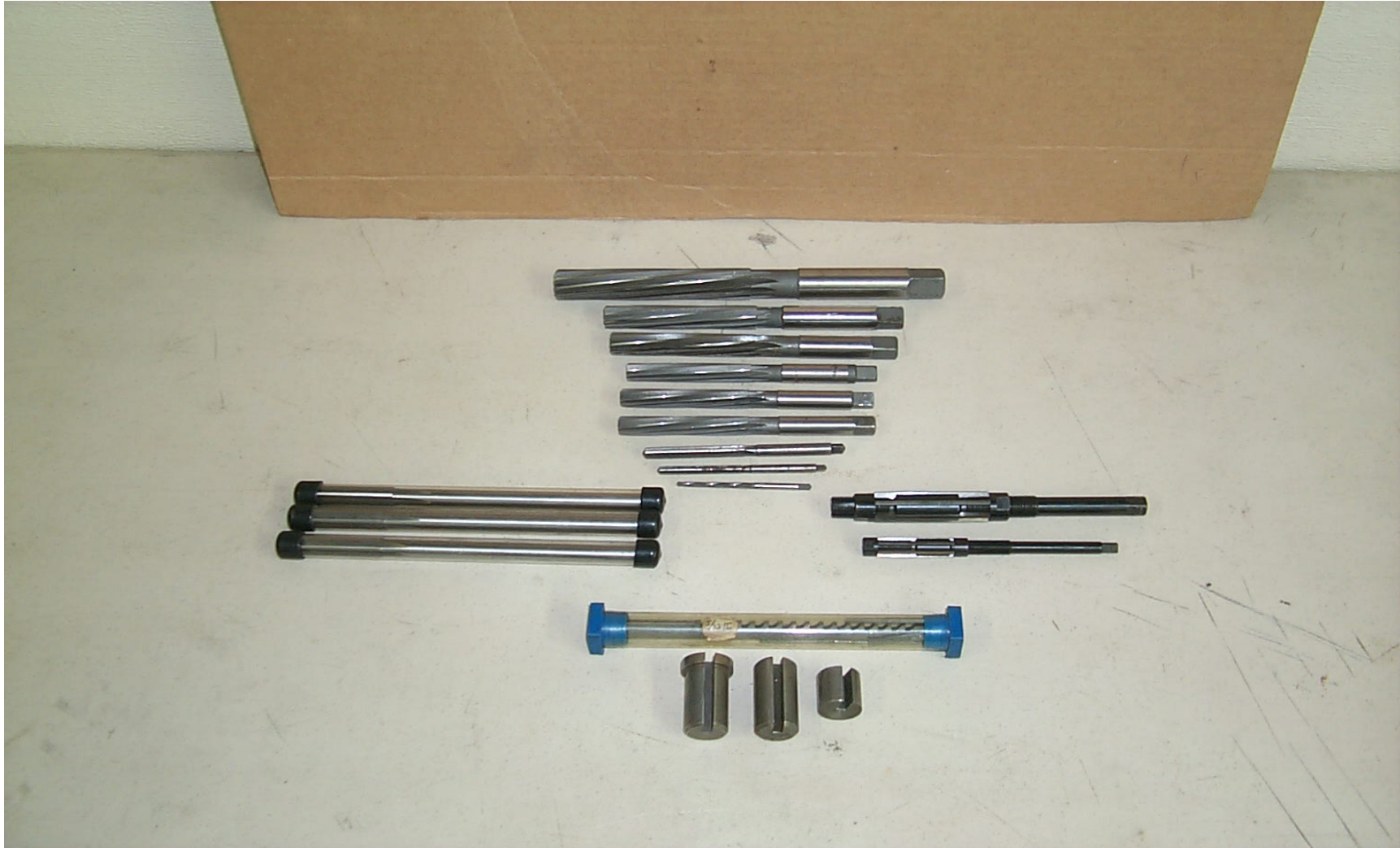
SPIRAL FLUTE HAND REAMERS (7/8", 21/32", 5/8", 13MM, 1/2" (2) & 0); STRAIGHT FLUTE HAND REAMERS (5/16" & 7/32"); MACHINE REAMERS (.502" 503" & .504"); ADJUSTABLE REAMER (23/32"-25/32" & 15/32"-17/32"); 7/8" ID FOR 5/32" KEYWAY PRESS BROACH
