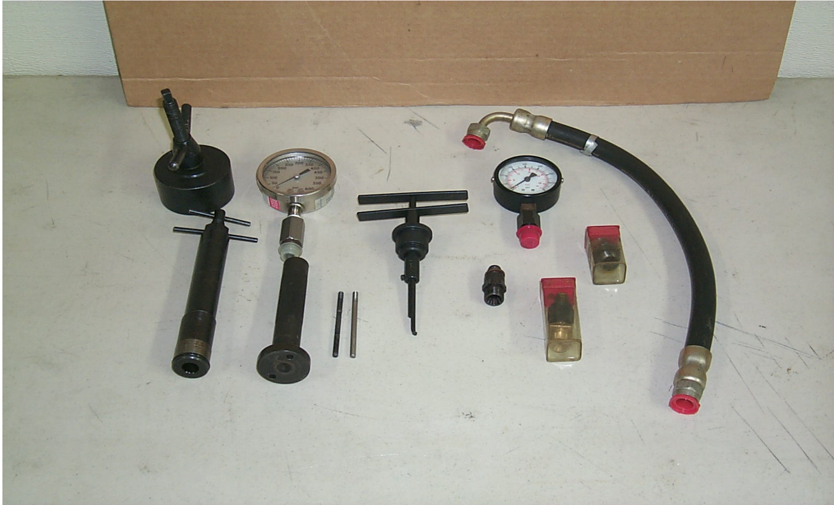
OIL PUMP REMOVER (18G183): SCREW IN OIL PRESSURE GAUGE (SCREWS INTO OPERATING VALVE RETAINER CAP BORE): ACCUMALATOR PISTON HOUSING REMOVER (18G182): OIL PUMP INSTALLER ((18G184): "J" TYPE OIL PRESSURE RELIEF VALVE REMOVER (LH401A): OIL PRESSURE GAUGE 0-800PSI (18G251 WITH VARIOUS ADAPTORS):
