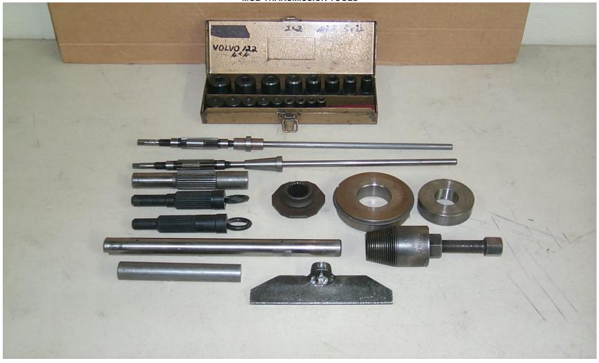
UNIVERSAL CLUTCH ALIGNMENT TOOL: EARLY MGB TRANSMISSION CASE REAMER SET (USED FOR REAMING TRANS CASING FROM .643" - .668" OD TO ACCEPT LATER SIZE OD LAYSHAFT: CLUTCH ALIGNMENT TOOLS (MGB EARLY. MGB LATER & MGA: INPUT SHAFT SPLINED HOLDER: INPUT SHAFT BEARING SPACER: REAR MAINSHAFT BEARING SPACER: DUMMY LAYSHAFTS: REAR TRANSMISSION OIL SEAL REMOVER: DRAIN PLUG ADAPTOR (SCREW INTO DRAIN PLUG HOLE & HOLD IN VISE JAWS. SUPPORTS TRANSMISSION):
