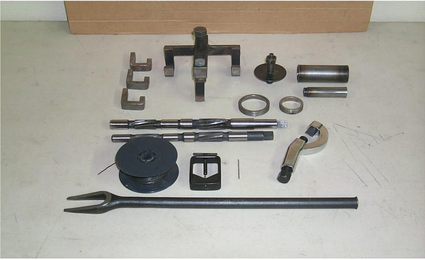
MGB LTD ED STEERING WHEEL PULLER (STILL REQUIRES EXTRA EFFORT. KEEP PULLER STRAIGHT & LEVEL AT ALL TIMES. USE IMPACT WRENCH): GREASE CAP REMOVER: KING PIN LOWER BUSH REMOVER SET (APPLY HEAT ON THIS OPERATION): HUB BEARING TRACK INSTALLATION RINGS: MGB KING PIN REAMER: MG MIDGET KING PIN REAMER: NUT SPLITTER: BOLT & NUT WIRING ANVIL KIT: TIE ROD END REMOVER:
