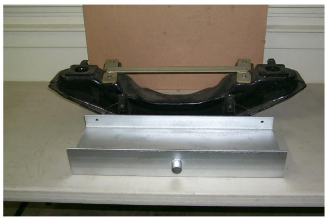
IN THE ABOVE IMAGE WE SHOW A NEW MGB CROSSMEMBER WITH MY FRAME CHECKING JIG PLACED INTO POSITION. THIS JIG WILL ALLOW YOUR USED CROSSMEMBER TO BE CHECKED FOR STRAIGHTNESS. IF YOUR FRAME HAS TO BE STRAIGHTEN, USE THE JIG FOR CHECKING THE ACTUAL FRAME FOR ACCURACY. (IT IS NO USE TRYING REINSTALL THE CROSSMEMBER IF THE FRAME IS OUT OF WHACK). NOTE: ENGINE HAS TO BE REMOVED FOR THIS SECOND OPERATION
