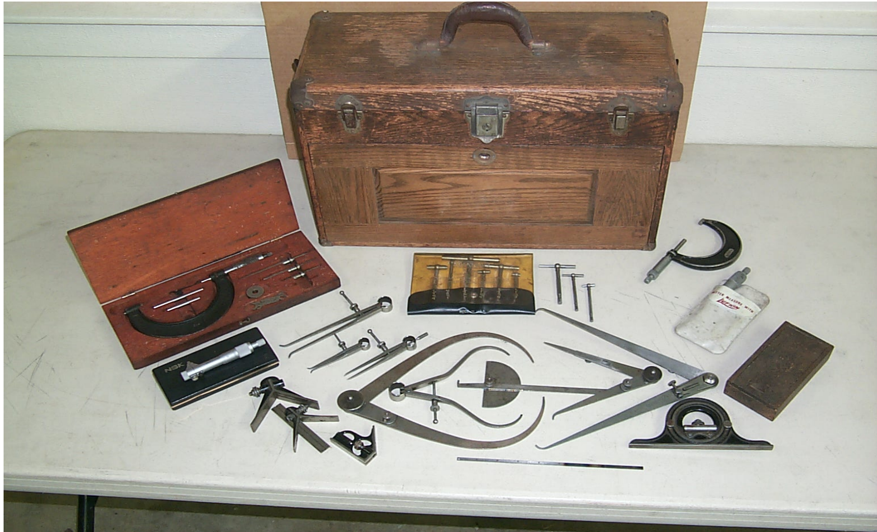
ORIGINAL MACHINIST TOOL BOX: MICROMETER SET (0-4") : SNAP GAUGE SET (1/2"-6") ADDITIONAL SNAP GAUGES: MICROMETER (2"-3") MICROMETER (1"-2") MICROMETER (0-1") : INSIDE MICROMETER (0-1") : VARIOUS MACHINIST MEASURING TOOLS:
