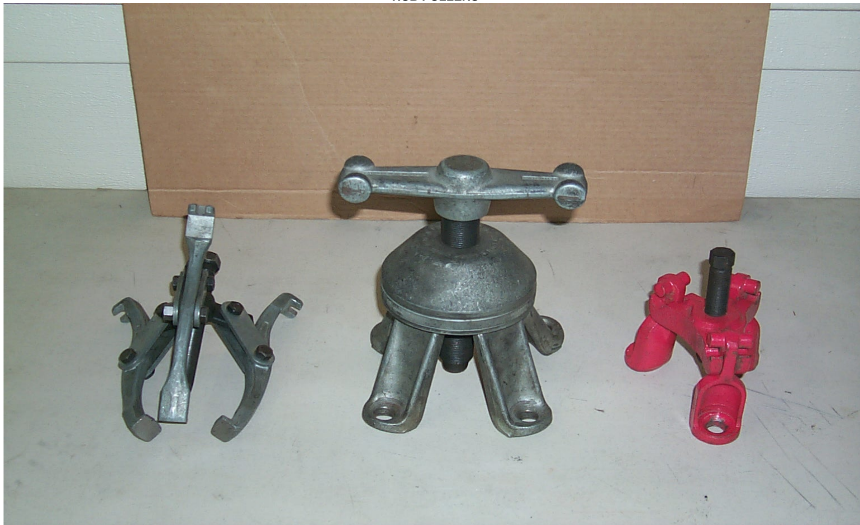
3 - LEGGED PULLER (SLOTTED END WIDTH 3/8"): 4 - LEGGED HEAVY DUTY PULLER (HOLE SIZE 11/16"): 3 - LEGGED PULLER (HOLE SIZE 9/16")
