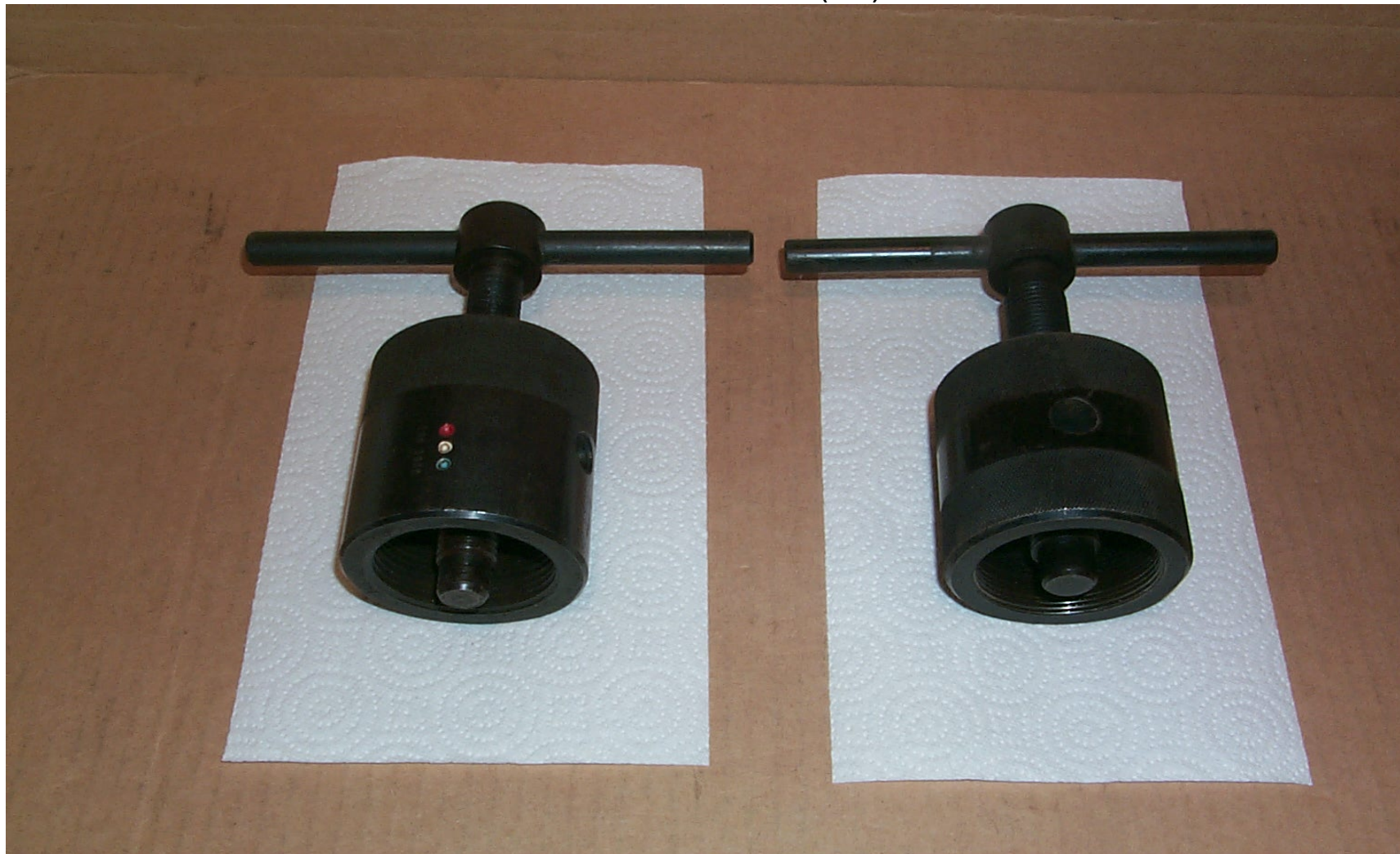
MGA & MGB WIRE WHEEL HUB FINE THREAD (18G363): MGB WIRE WHEEL HUB PULLER COURSE THREAD (18G1032)
