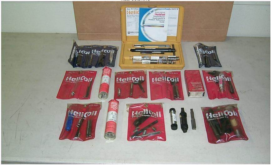
M6 X 1 KIT (2 KITS): 14mm SPARK PLUG THREAD REPAIR KIT: M10 X 1.25 KIT : USS HELI-COIL KITS (8-32: 10-24: 1/4" X 24: 5/16" X 18: 3/8" X 16: & 7/16" X 14: SAE HELI-COIL KITS (1/4" X 28: 5/16" X 24: 3/8" X 24: 1/2" X 20: & 5/8" X 18:
