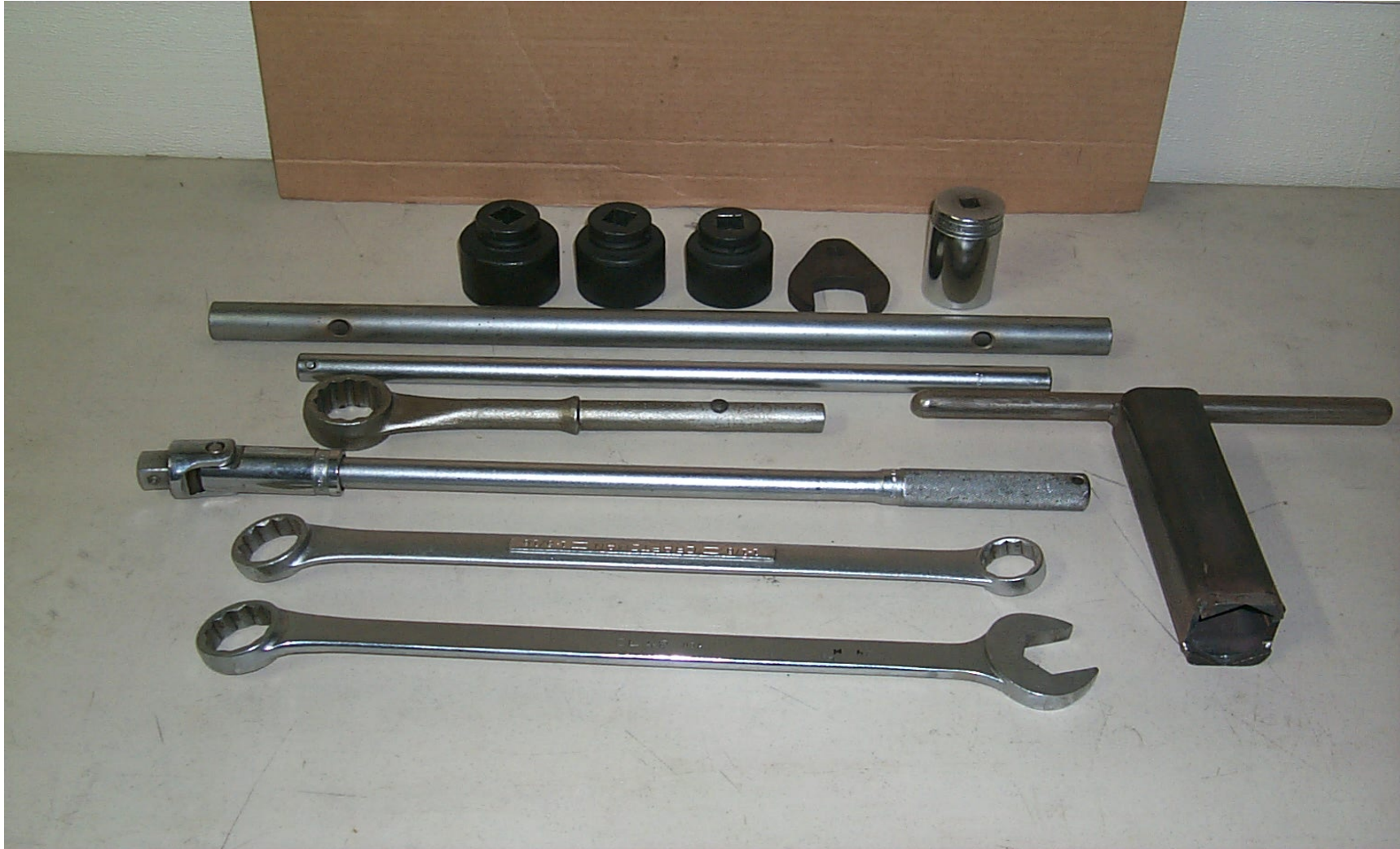
SNAP-ON IMPACT HEAVY DUTY SOCKETS (1.5/8" 1.11/16" & 1.13/16" ALL 3/4" DRIVE): 1.5" CROW FOOT SOCKET (1/2" DRIVE 18G1182): 1.5" DEEP SOCKET (1/2" DRIVE): 1.5" BOX END WRENCH WITH INNER & OUTER EXTENSION BARS: BREAKER BAR (3/4" DRIVE): 1.1/8" X 1.5/16" BOX WRENCH: 1.5/16" COMBINATION WRENCH: TUBE WRENCH (1.7/8" SIZE ACROSS FLATS)
