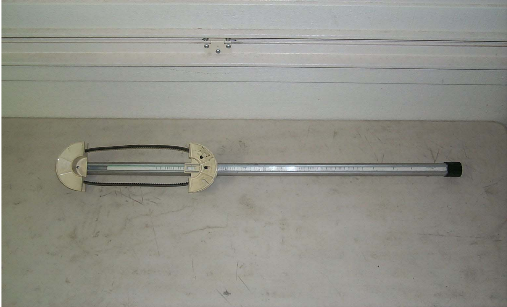
FAN BELT CHECKING GAUGE (1/4" 5/16" 3/8" 1/2" 5/8" 11/16" 3/4" 7/8" & 1' WIDTHS)
