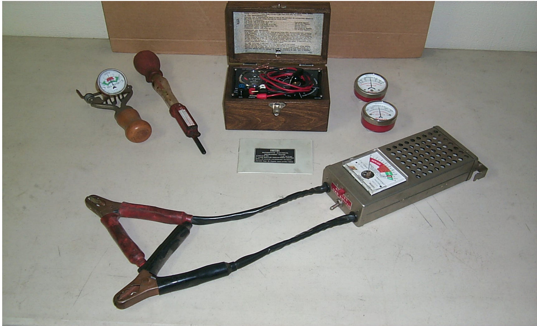
OLD STYLE 6 VOLT BATTERY CELL LOAD TESTER: HYDROMETER: SMITHS ELECTRICAL AUTOMOTIVE INSTRUMENT TESTER (BLT005001): INDUCTION AMP GAUGES (0-75AMPS) & (0-600AMPS): HAND HELD BATTERY LOAD TESTER (6V & 12V)
