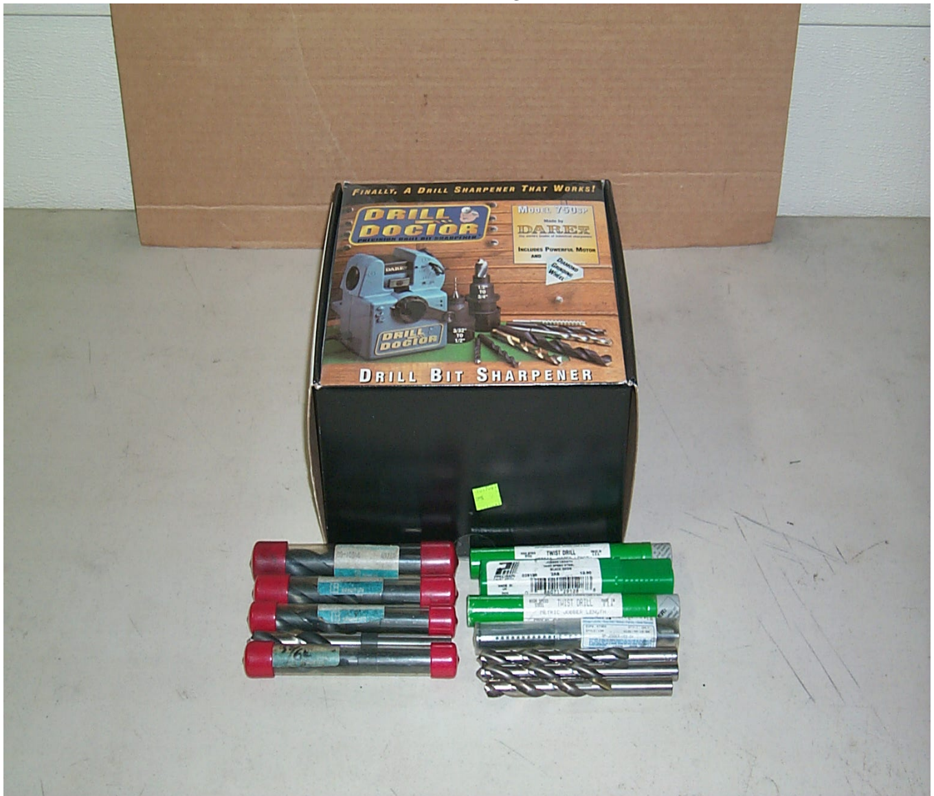
1/2" SHANK DRILL BITS (49/64" 41/64" 37/64" 35/64" & 33/64") DRILL DOCTOR (EARLY VERSION) DRILL SIZE SHANK DRILLS (12.90mm- 12.80mm x 3- 12mm x 2 & 11.2mm)
